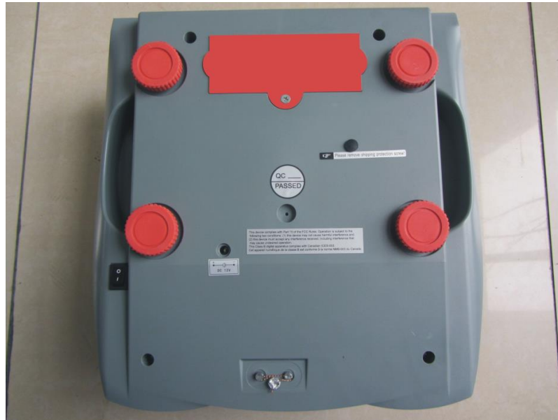
Figure 2 Sealing of A31P with wire and seal.
